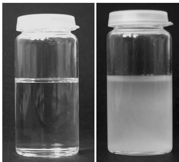
Fig. 1 Suspensions of nanoscale \text{Mg}(\text{OH})_2 in DEG: \varnothing = 20 \text{ nm} , 2.9 mg/ml (left); \varnothing = 100 \text{ nm} , 2.9 mg/ml (right)
